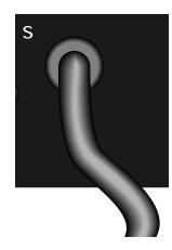
S. SUPPLY CORD - This is a grounding type supply cord to reduce the possibility of shock hazard. Completely unwind the cord from its cord wrap to prevent blocking air flow to the transformer. Be sure to connect the cord to a grounded receptacle. DO NOT ALTER THE AC PLUG.
